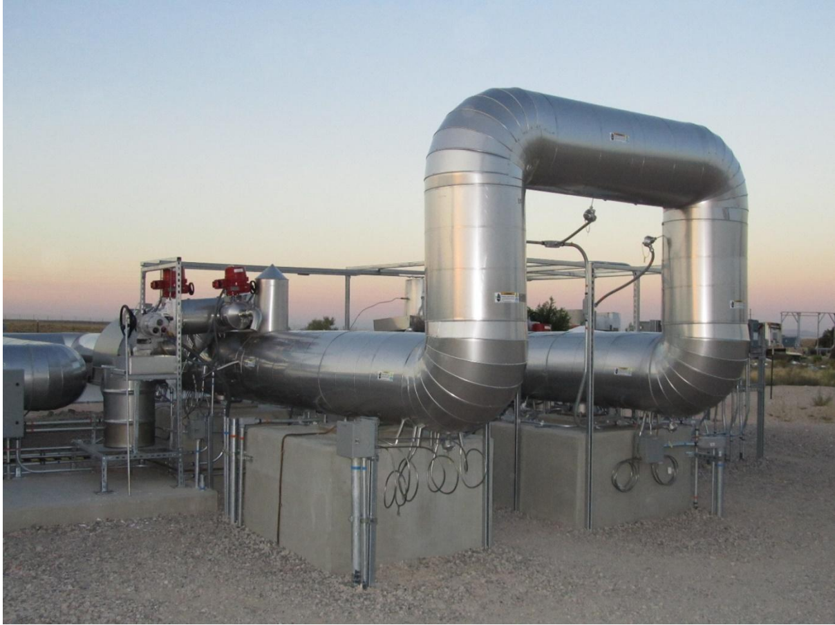
Figure 130. Test loop experiment section for the molten salt test loop [105].
