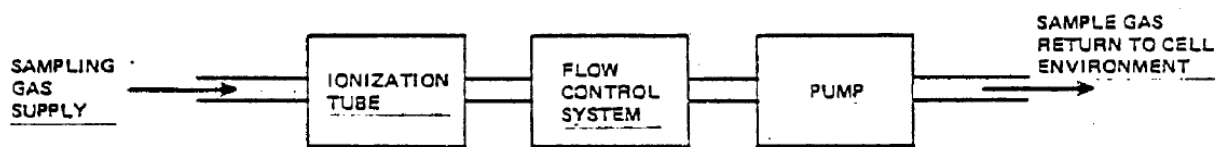
Figure 70. Surface ionization monitor for particulates.
