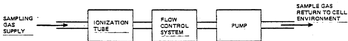
Figure 25. Surface ionization monitor for particulates (SIMP) diagram.
