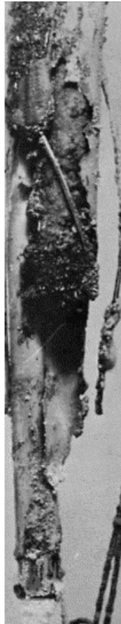
Figure 86. Partially melted fuel elements. [57]
