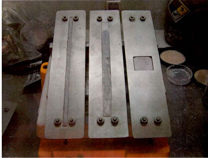
Figure 41. Slits between stainless steel plates used for sodium testing [39].
