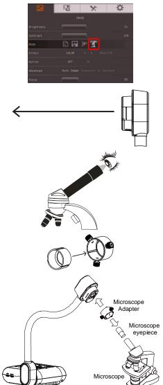
Make sure the arrow on the camera head and microscope adapter are on the same side to connect and twist clockwise for the arrows to meet and lock.
