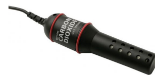
Figure UII-3. \text{CO}_2 sensor. Keep the sensor upright at all times.
